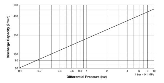
1. Differential pressure is the difference between the inlet and outlet pressure of the air vent. 2. Capacities are equivalent capacities of air at 20 °C under atmospheric pressure.
